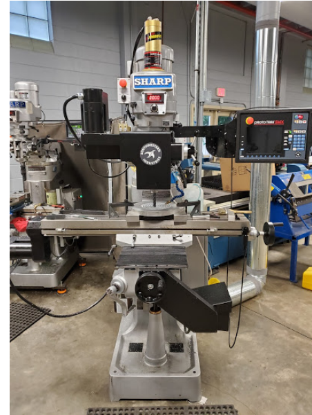
Sharp Knee Mill w/ ProtoTrak CNC
