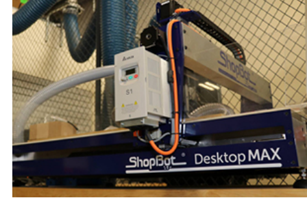
Shopbot Desktop MAX router X: 965mm; Y: 635mm; Z: 140mm
