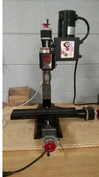
Sherline vertical mill X: 220mm; Y: 228mm; Z: 159mm
