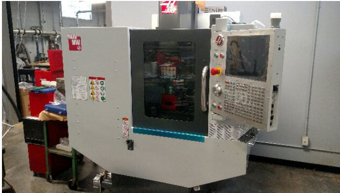
HAAS Minimill-EDU VMC X: 406mm; Y: 305mm; Z: 254mm
