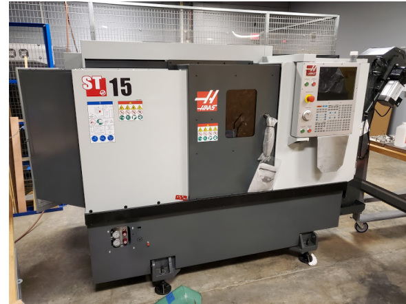
HAAS ST15 CNC Lathe (20hp) L: 406mm, Dia: 419mm
