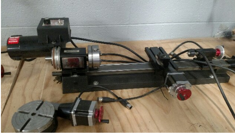
Sherline CNC Lathe (0.08hp) L: 430mm, Dia: 90mm
